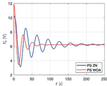
Figure 6. Simulated control signals for proportional-sum controllers
