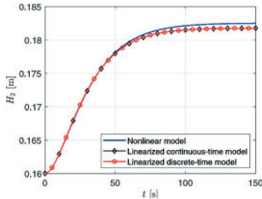
**Figure 2.** Continuous-time and discrete-time linear model accuracy against nonlinear plant behavior
