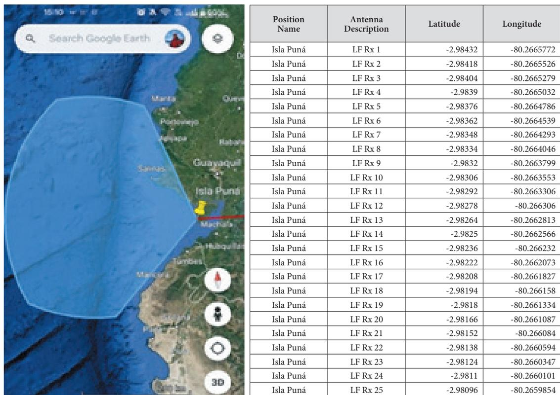
Figure 5. The simulated coverage area by one HFSWR (left), and corresponding antenna positions (right)
