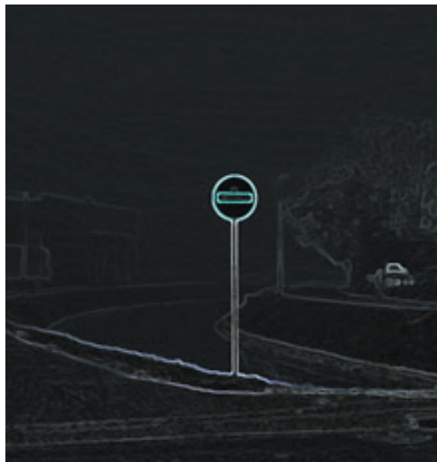
Figure 4. Edge Detection in Image Processing
