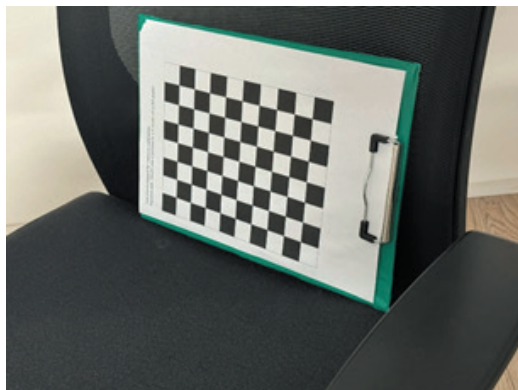
Figure 3. Checkerboard for lens calibration.
