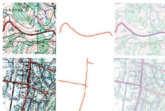
Figure 4 - Presentation of methodology steps and positional accuracy of roads (Map segment – left, Road extraction map – Middle, Road vector data – right).
