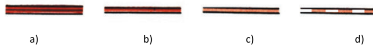
Figure 1 - Symbol for highway (a), asphalt road wider than 6 m (b), asphalt road from 3 to 6 m (c) and macadam road (d).
