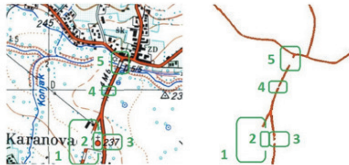
Figure 2 - View of the map segment (left) and the corresponding extracted imageroads (right) with appropriate markings.
