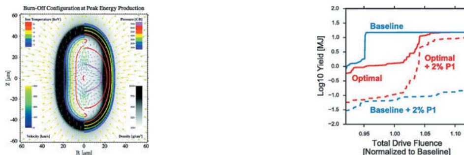
Figure 3 - (left) Velocity (arrows), density (gray), ion temperature (left color contours), and pressure (right color contours) at the time of peak energy production for an ovoid implosion. (right) The surrogate's estimate of yield under changing total drive fluence for the baseline (round) and optimal (ovoid) cases. Reproduced from [20], with the permission of AIP publishing.
