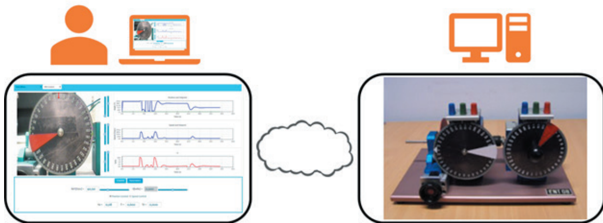
Figure 1 – Basic architecture of a weblab.
