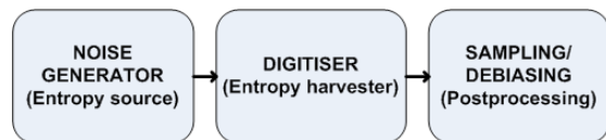
Fig. 2. TRNG operation block diagram
